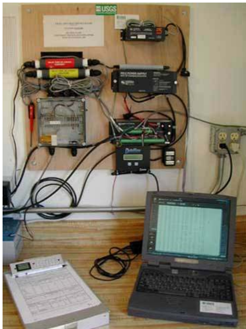
Anacostia River real-time sampling equipment on the Northeast Branch at Riverdale, MD
